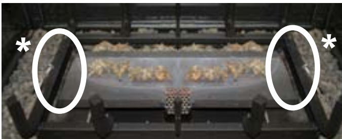
Figure 26. Place the provided embers in the 5 pronged ember holders. Be sure to not directly cover any of the burner holes.
