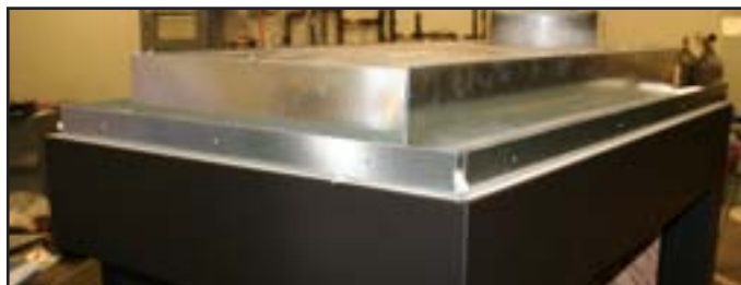
Figure 7c. Finished removing Nailing Flange extension.
