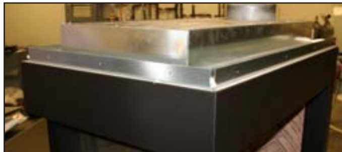
Figure 7c. Finished removing Nailing Flange extension.
