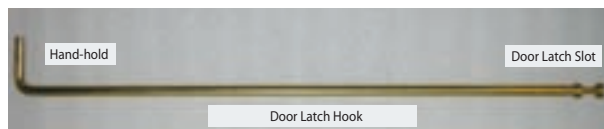
Figure 27b. Door buckle Tool
