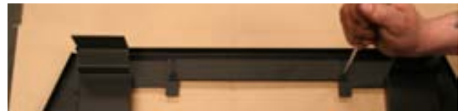
Figure 10a. Pull the air baffle forward as far as possible and screw the air baffle closed.
